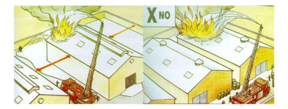
The site layout designed to allow possible separation of incompatible materials by use of separate buildings, fire walls or other acceptable precautions should permit safe movement and transport of materials; it should have sufficient space to give reasonable working conditions and allow clear access from two sides.
