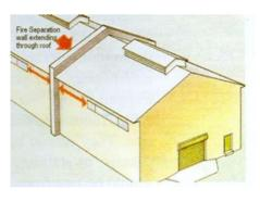
mineral wool or glass fibres. Internal division walls, designed to act as fire breaks, must provide at least *one hours resistance* and should rise to a height of one metre above the roof or have other means of preventing a fire from spreading.
