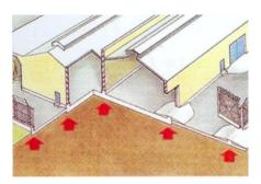
of spillage is high, there should be a separate drainage system with sloped floor, a bund and a collection sump.
