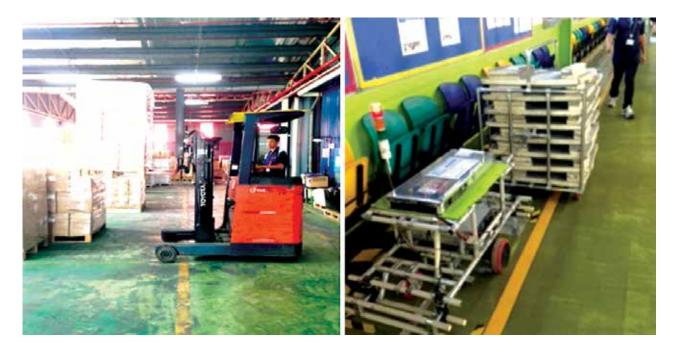
Figure 6.5: A powered-reach truck is used to move and lift materials short/long distances (Left). A tugger AGV used for pulling trolleys loaded with heavy objects between workstations (Right)
