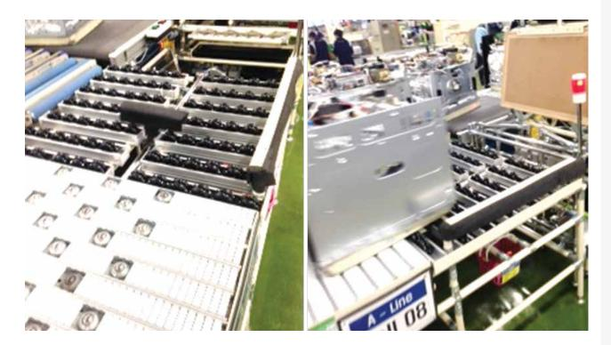
Figure 6.3: An assembly line embedded with roller tracks and ball bearings allows heavy objects to be turned and repositioned
