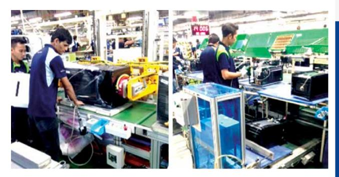
Figure 6.4: Auto-clamping lifter used to lift up/down and turn products (Left) and a hydraulic-cylinder lifter allows products to be lowered and pushed into transferring conveyor by means of a foot-switch (Right).
