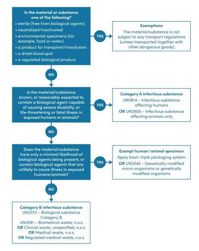
Figure 6.2 Classification of infectious substances for transportation
