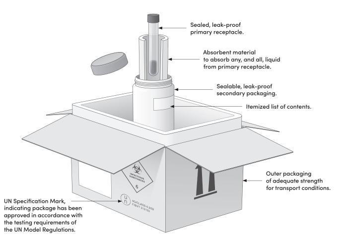
**Figure 6.4** Example of triple packaging materials suitable for Category A infectious substances
