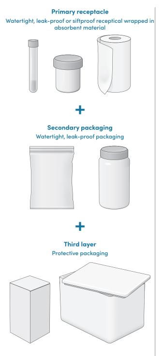
**Figure 6.3** Example of triple packaging for infectious substances
