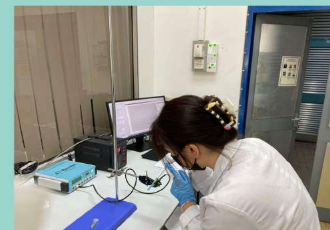
Figure 1: Electrochemical biosensing of exosomes using a potentiostat.
